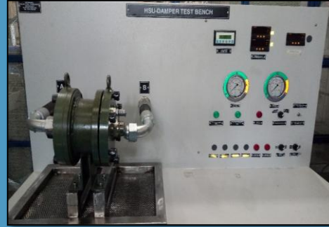
Test rig for plotting Flow Vs Pressure across Dampers
