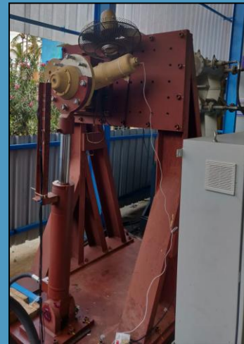
PLC integrated test setup to carry out 500,000 cycles of endurance test
