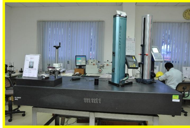
Surface Table 00 Grade for calibration
