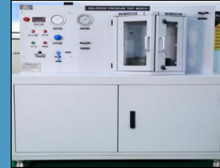
Proof pressure test rig for 1000 Bar
