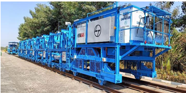
Track Slab Laying Car
