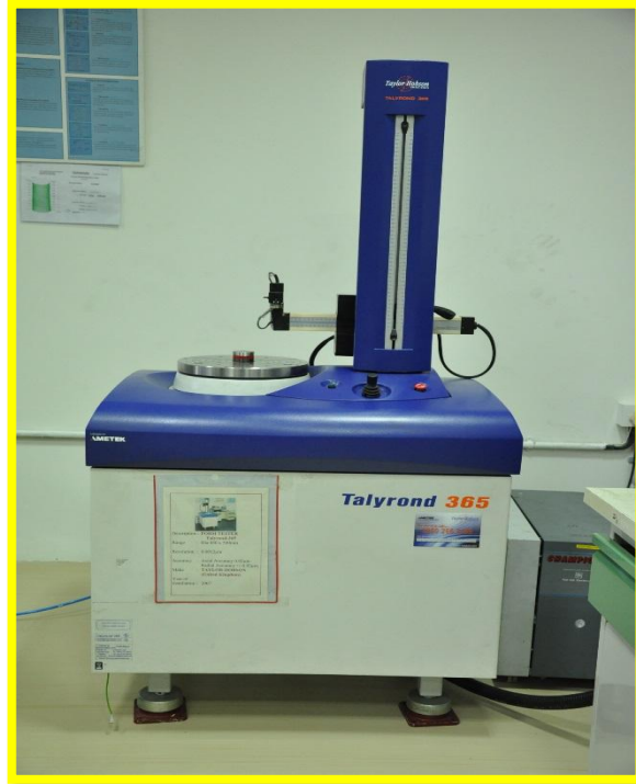
Form tester for Roundness, Cylindricity of super finished parts
