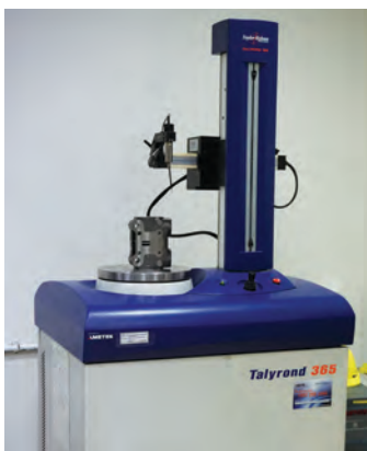
Form tester for Roundness Cylindricity, Straightness of super finished parts
